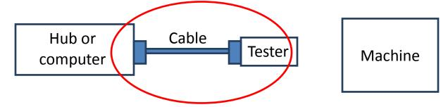
Test 3 With tester still plugged into cable, plug tester & cable into machine Both lights should turn on and they should be the same color (but they may be red or green)
